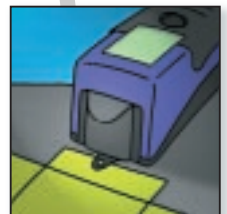
Color measurement of original reference materials with the SpectroEye
